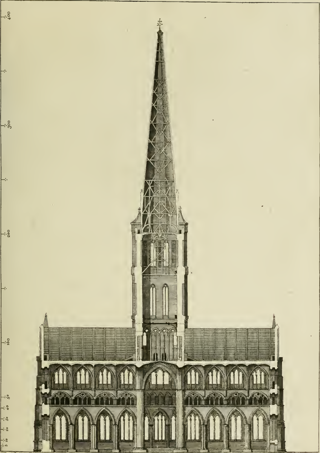
A Section of the Church, with the Tower and Spire? Shewing the Critical Mechanism of the whole Structure?
